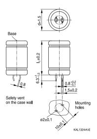
Snap-in terminals, length (6.3 + 1/-1.5) mm. Also available in a shorter version with a length of (4.5 - 1.5) mm. Marking by an adhesive label.
