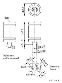
Snap-in capacitors are also available with 3 terminals (length (4.5-1.5) mm). Marking by an adhesive label.
