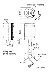
Snap-in terminals, length (6.3 + 1/-1.5) mm. Also available in a shorter version with a length of (4.5 - 1.5) mm. Without insulation sheet at the base.
