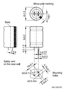
Snap-in capacitors are also available with 3 terminals (length (4.5-1.5) mm). Without insulation sheet at the base. PET insulation is marked with label "PET" on the sleeve.
